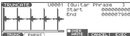
5. If you want to replace the current sample with the truncated sample, press [F4 (OVER WRITE)] to display the "✓" mark.
