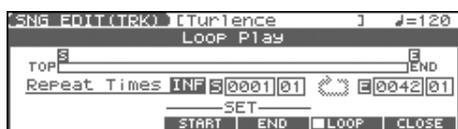
3. Move the cursor to the desired parameter, and use the VALUE dial or [INC] [DEC] to make the setting.
