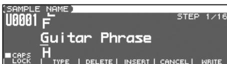
If you have selected more than one sample, a message will ask you to confirm the writing operation. Samples will be written into the identical number corresponding to each bank of the sample list. Sample names will be assigned automatically. If you want to write the samples, press [F6 (EXEC)]. If you decide to cancel, press [F5 (CANCEL)].
