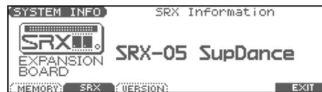
\* If the name of the board does not appear, it is possible that the board is not being recognized correctly. Turn off the power as described in **Turning Off the Power** (p. 16), and re-install the Wave Expansion Board correctly.
